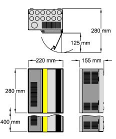
SCS0420 D version - 400x220x155mm RCBO & RCBOX version - 340x255x155mm
