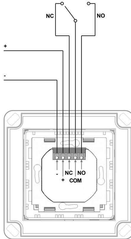
To switch from more than one position simply wire two or more units in parallel to achieve two way and intermediate switching.
