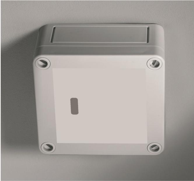
The MPD-C-EXT 12-24V microwave presence detector switch is designed to provide automatic control of lighting, heating or ventilation loads. It detects movement using a highly sensitive microwave detector. This works by emitting low power microwave signals and measuring the reflections as the signals bounce off moving objects. The MPD-C-EXT 12-24V is optimised for ceiling mounting applications to give detection over long distances.
