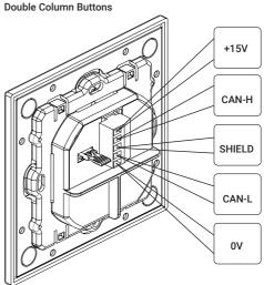
Maximum segment distance: 500m (1640 ft) Devices per segment: 100 (without bridge or repeater)
