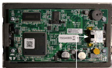
CAT5, RJ45 Connection to HVAC-1
