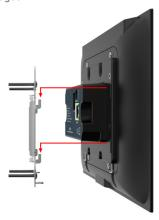
Tighten the 2 captive screws to secure the TSE80-B to the mounting bracket
