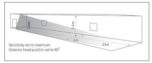
Ideal for corridor or aisle applications. Maximum recommended mounting height: 3m
