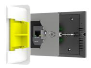
Tighten the 2 captive screws (one at each side) to secure the TSE55-B to the mounting bracket.
