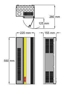
SCI1205 D version - 690x220x155mm RCBO & RCBOX version - 550x255x155mm
