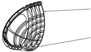
Lateral tear pattern for making a 'slot' style detection shape
