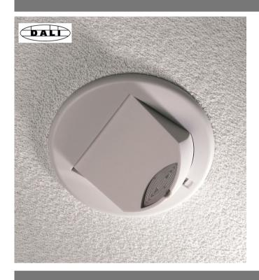
The MPAD-C-A-DALI-230V microwave presence detector provides automatic control of lighting loads with optional manual control. The MPAD-C-A-DALI-230V detects movement using a highly sensitive microwave detector. This works by emitting low power microwave signals and measuring the reflections as the signals bounce off moving objects.
