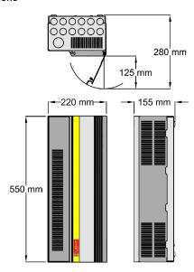
SCS1220 D version - 690x220x155mm RCBO & RCBOX version - 550x255x155mm
