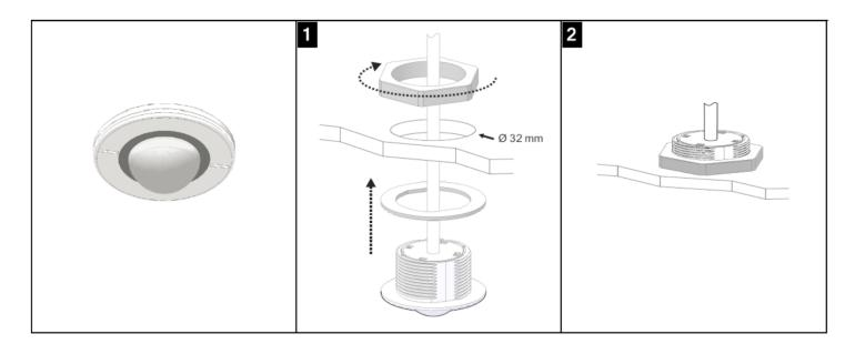
The PPAD-C-MB-EXT-DALI-ADDR IS supplied with 1m, 2 core 1.5mm<sup>2</sup> double insulated cable to connect to the iLight DALI Network - SCMD2/4. The device is designed to operate correctly polarity-free.
