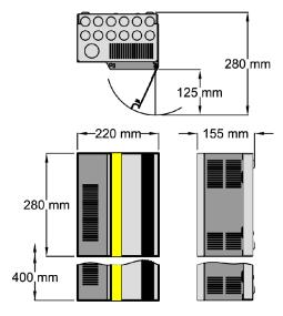
SCH0410 D versions - 400 x 220 x 155mm SCH0410 RCB0 & RCB0X versions - 340 x 255 x 155mm
